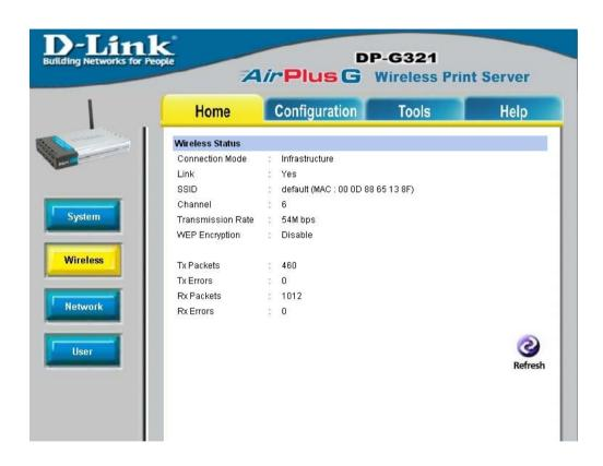
**Wireless Status:** The items in this field display information about the wireless LAN, such as the connection mode (Infrastructure or Ad-Hoc), SSID, channel, data transfer rate, WEP encryption, and the packets status.
